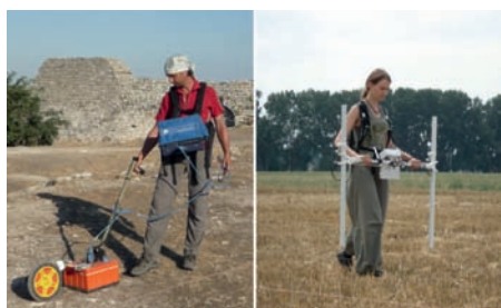
Ground Penetrating Radar and Geomagnetism in the field. Both instruments are supplied by TOPOI and used in many projects
