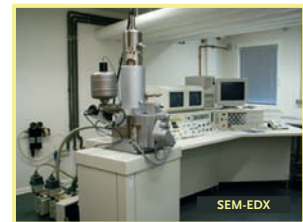
Fig. 5: The Scanning-Electron-Microscope with Energy-Dispersive-X-ray detection
